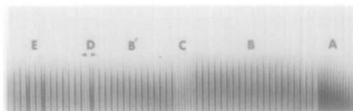
FIG. 1. Electron micrograph of a crystal showing mixed intergrowth of \beta - and \beta'' -alumina. A and C mark the \beta'' -alumina parts while B and B' are \beta -alumina. D and E mark disordered regions.
